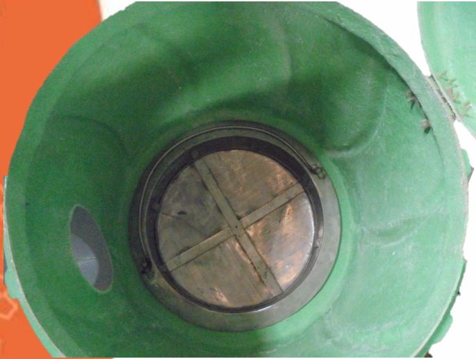
INWARD SECTION: ABOVE SS FILTER
